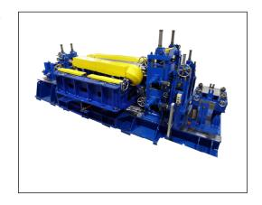
developed and brought many unique technologies into this industry like "FFX Mill" and "Roll Box", which apply common-use roll technology and have high formability for quality round & square pipe production. Especially, nearly 50 sets of FFX Mill have been installed during the past ten years since its development, which make it win worldwide clients' full confidence on the best pipe forming mill currently available in the world.
